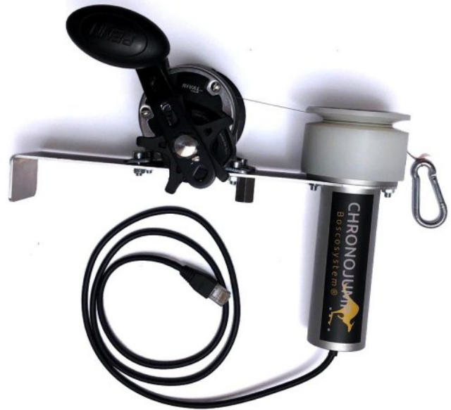
(Encoder, electronic and cables)
